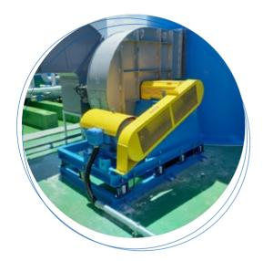
A fan is a device that creates air flow and applies pressure to move gas through the impeller. When resistance to corrosion and chemicals is required due to chemical substances, FRP material is used. For high-temperature or abrasive air intake conditions, metals such as SS 400 or STS 304 are used for manufacturing.
